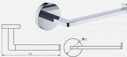
Zinc alloy base + stainless steel tube, chrome plated
