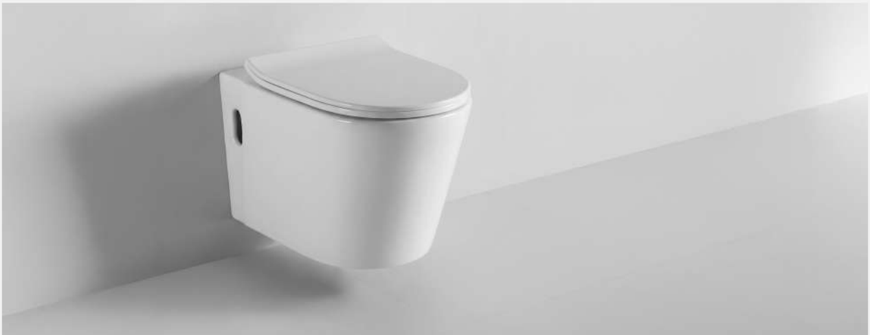
8539W Wall Hung Toilet Size: 570*350*365 MM P-trap: 180mm Roughing in
